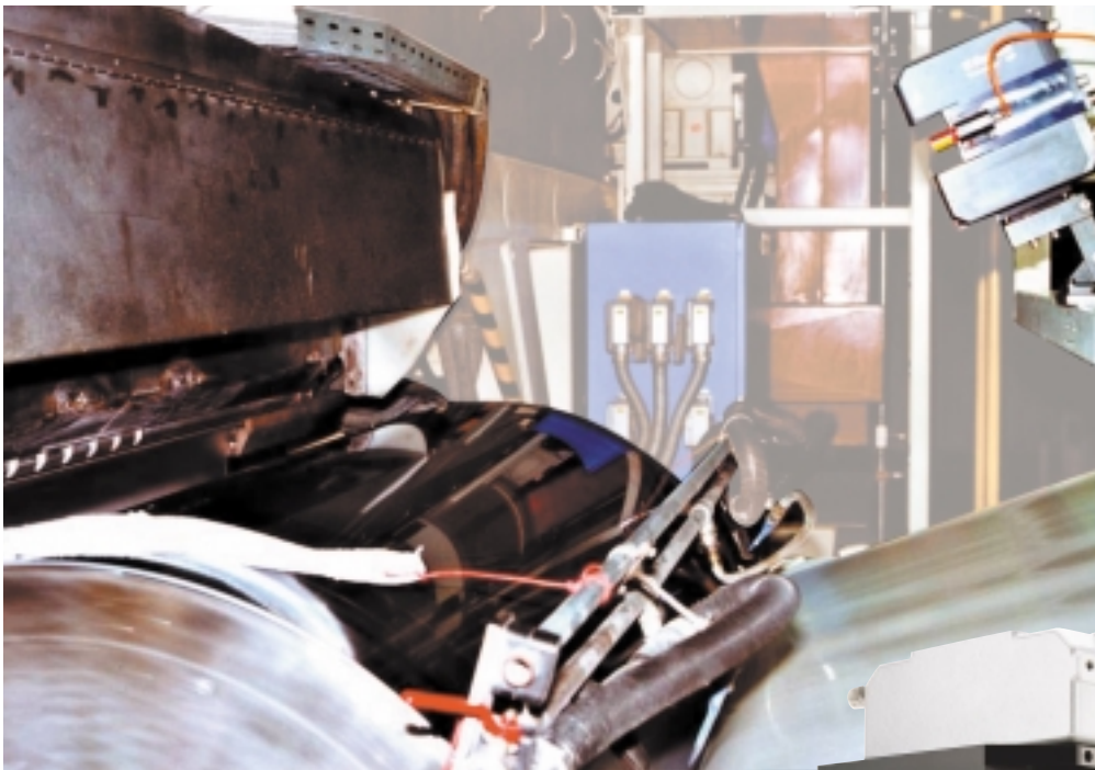
The EC100 provides real time temperature analysis for extrusion coating processes. (Photo: Courtesy of SIG Combibloc GmbH, Wittenberg, Germany)
